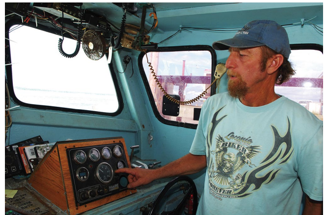
Capt. Neal Pike explains the important relationship between engine RPM, speed and GPH/MPG readings from his FloScan unit in reducing fuel consumption and operating overhead.
